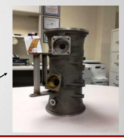
Weight: 11.25 lbs (5102.91 g) Height: 13.75 in (349.25 mm) Typical Wall Thickness: 0.12 in (3.04 mm) Material: Inconel 625 Nickel Base; AMS 5402 Application: Aircraft Engine; Exhaust Outlet Tube.
