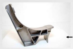
Weight: 1.85 lb (839.14 g) Height: 5.75 in (146.05 mm) Typical Wall Thickness: .08 in (2.03 mm) Material: 17-4PH Stainless Steel; AMS 5342 Application: Aircraft Engine; Bumper-Lower Section.
