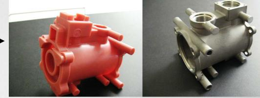
Weight: 3.05 lb (1383.45 g) Height: 7.00 in (177.80 mm) Typical Wall Thickness: .25 in (6.35 mm) Material: 347 Stainless Steel; AMS 5362 Application: Aircraft; Hydraulic Pump (Wax & Machined Casting).
