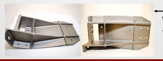
Weight: 2.50 lb (1133.98 g) Height: 8.35 in (212.09 mm) Typical Wall Thickness: .09 in (2.28 mm) Material: 17-4PH Stainless Steel; AMS 5344 Application: Aircraft Engine, Nacelle; Fitting-Latch.
